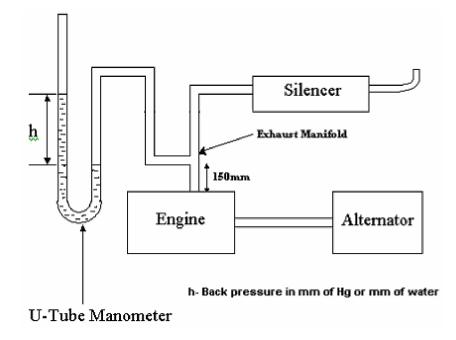
Back Pressure should be measured at 100 % loading condition
